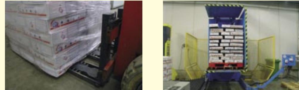
is much cheaper. Manual handling is also possible but this will increase labour costs. The replacement of a standard pallet by a pallet with extra supporting laths makes it possible to place boxes directly on the forks. A third RollerFork® in the middle supports the inner layer of boxes. For standard pallet handling the middle RollerFork® can be folded upwards.
