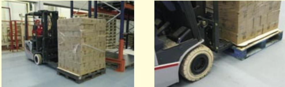
The plastic RF-Pallet, on the other hand, is only used inside the production area and can save you a lot of money. The pallet has an extra set of synthetic slats on the upper deck and the RollerForks® perfectly fit between them. By first laying a slip-sheet on the pallet, the forks later roll effortlessly under the slip-sheet. After the goods are on the RollerForks® they simply roll off the forks on a standard wooden pallet inside the warehouse where the wooden pallet can be stored.
